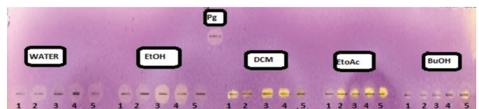
Figure 1. Antioxidant capacity by qualitative DPPH test on TLC of Ononis species 1: O. basiadnata root extract, 2: O. basiadnata herb extract, 3: O. sessilifolia root extract, 4: O. sessilifolia herb extract, 5: O. macrosperma herb extract, Pg: Propyl gallate
