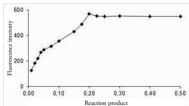
Figure 3. Effect of dansyl chloride volume on reaction efficiency (0.5  $\text{mg}\cdot\text{mL}^{-1}$ )
