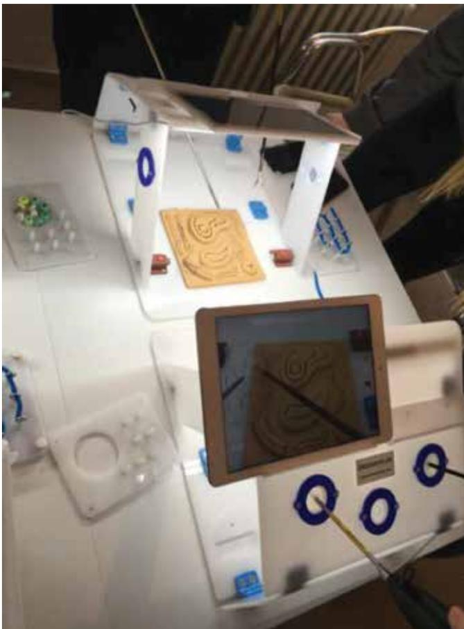
**Figure 1. Structure of the laparoscopy simulator**
