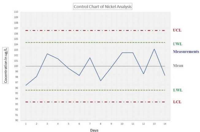
**Figure 2. Control charts of nickel by GFAAS. The concentration of nickel is presented in ppb while UCL, UWL, LWL and LCL stand for upper control limit, upper warning limit, lowest warning limit and lowest control limit, respectively. The blue line represents the stability in the nickel concentrations quantified among days**
