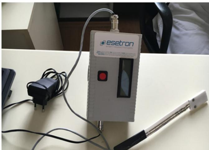
**Figure 2:** Jaw bite force measurement device
