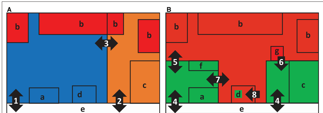
Figure 1. Schematics of the ICU and cardiology IMC before (A) and during (B) the first wave of the COVID-19 pandemic. (A) Blue, ICU; Orange, cardiology IMC; Red, areas with a potential for microbiological contamination; White, area outside of the ICU and IMC; (a) locker room, (b) patient rooms, (c) meeting rooms and offices, (d) material elevator, (e) hospital hallway; (1) entry and exit to the ICU, (2) entry and exit to the cardiology IMC, (3) passage between ICU and cardiology IMC. (B) Green, clean area of the COVID-19 ICU; Red, area of the COVID-19 ICU with a potential for microbiological contamination; White, area outside of the COVID-19 ICU; (a) locker room, (b) patient rooms, (c) break rooms, (d) material elevator, (e) hospital hallway, (f) changing area for personal protective equipment, (g) personal protective equipment removal area; (1) entries and exits to the (clean) COVID-19 ICU, (2) access to the contaminated COVID-19 ICU for staff/access to and exit from the contaminated COVID-19 ICU for patients, (3) exit from the contaminated COVID-19 ICU for staff, (4) supplies and sample gate to the contaminated ICU, (5) access from the contaminated ICU to the (clean) material elevator. ICU, intensive care unit; IMC, intermediate care unit; COVID-19, coronavirus disease 19.
