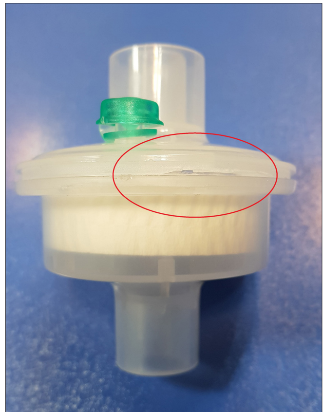
Figure 3. Cleavage of plastic fittings between two plastic parts of the HME filter HME: heat and moisture exchange
