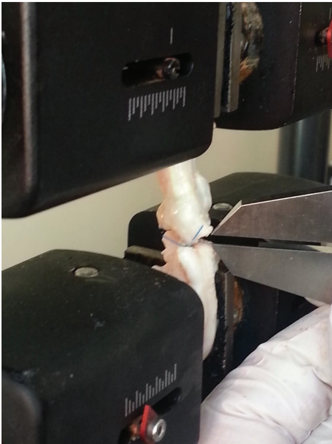
Figure 4. Photograph showing a sample mounted on the mechanical test device for biomechanical testing
