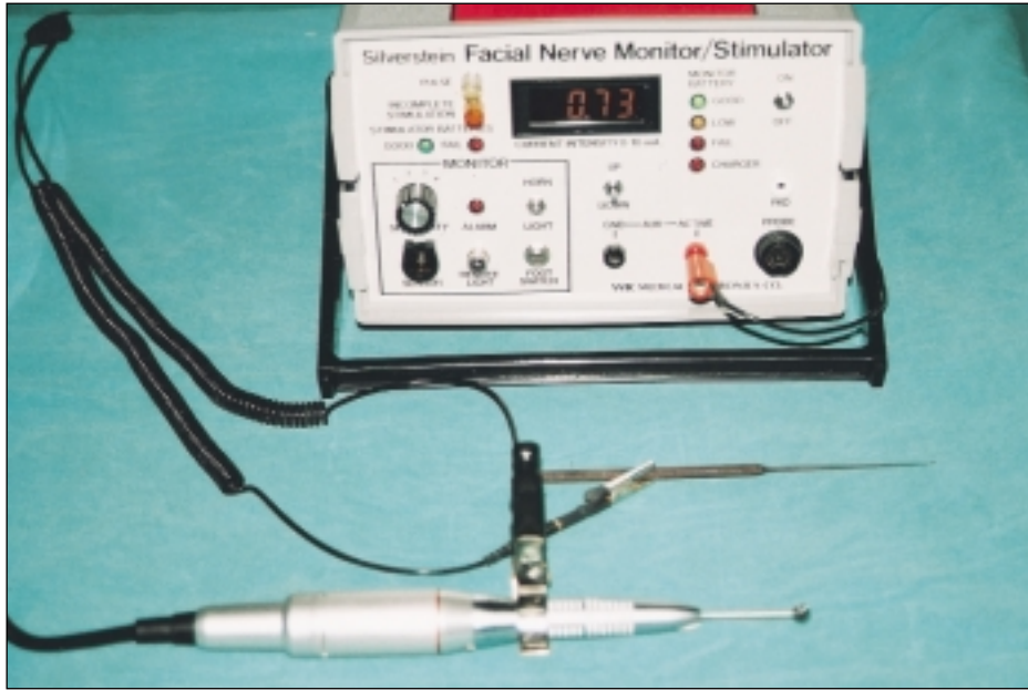
Figure 3. A drill was connected to one of the adapter's clip and a microsurgery device to the other clip.
