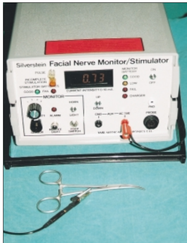
Figure 2. A hemostat-dissector was connected to the adapter clips for the parotid surgery.
