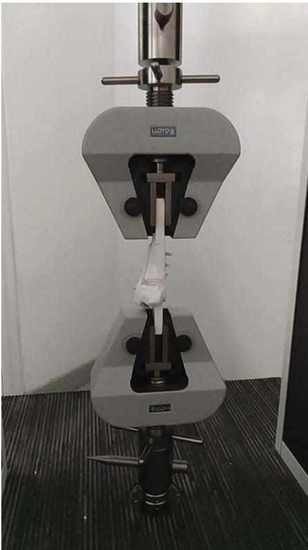
**FIGURE 3.** Tibia model with implanted plate on Llyod-Ametek EZ-50 Material Testing Machine.
